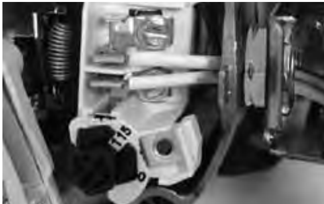
Figure 5: Voltage set to 115 volts, Dial Type
