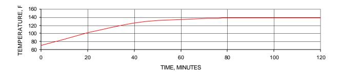
TYPICAL MOTOR SHELL T-RISE @ 40 PSI, 12V
