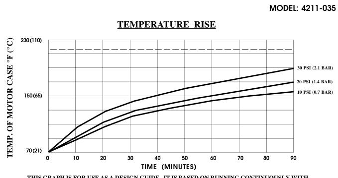
THIS GRAPH IS FOR USE AS A DESIGN GUIDE. IT IS BASED ON RUNNING CONTINUOUSLY WITH AN AMBIENT TEMPERATURE OF 70°F (21°C) IN STILL AIR. --- OPERATIONAL LIMIT.
