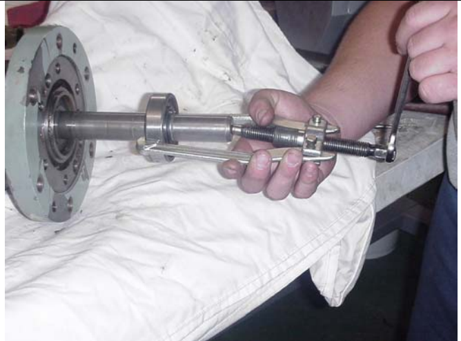
Use a puller to remove the bearing.
