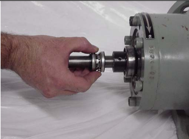
Remove the rotating part of the mechanical seal.
