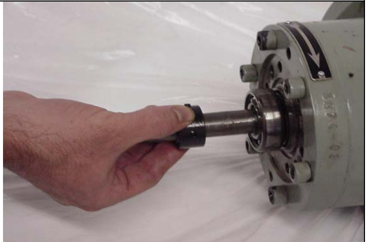
Loosen spacer setscrews and remove it.
