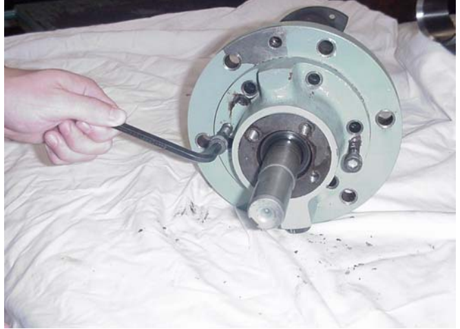
Remove the seal housing. Use 2 of the bolts as jackscrews to assist removal.
