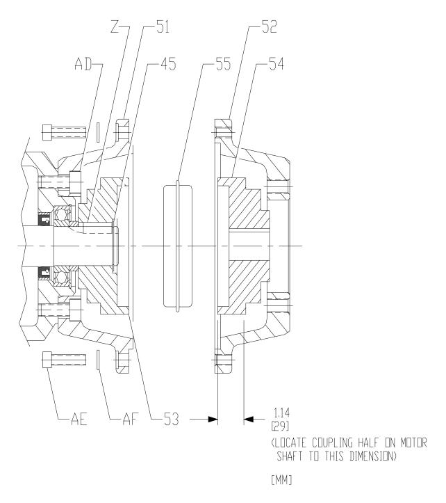
TYPE BHB HYDRAULIC DRIVE COUPLING ASSEMBLY FIGURE 7.3
