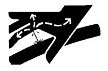
Injection Hazard: Do not try to stop a leak with your hand! Avoid any close contact with hydraulic fluid jets. Escaping fluid can penetrate skin, causing serious injury. In case of accident, see a doctor immediately for removal of fluid.
