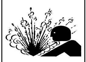
Over-pressure may burst pump or system components. Always include a relief valve in installation. Do not over pressurize pump or block discharge line while running.
