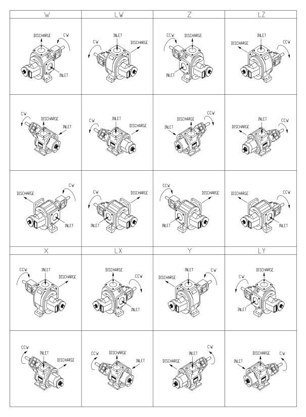
DIRECTION OF ROTATION FOR BHB PUMP CONFIGURATIONS USING THE RV STYLE RELIEF VALVE Figure B
