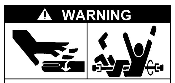
Operating without guards could result in serious injury or death. Machinery in operation can grab, crush, cut, mangle and dismember. Do not operate without adequate guards in place.
