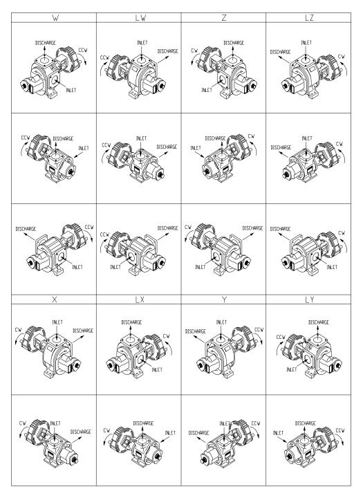
DIRECTION OF ROTATION FOR GHB PUMP CONFIGURATIONS USING THE RV STYLE RELIEF VALVE Figure A
