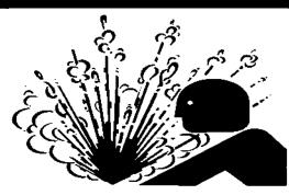
Over-pressure may burst pump or system components. Always include a relief valve in installation. Do not over pressurize pump or block discharge line while running.
