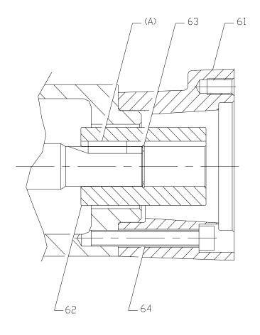
TYPE BH HYDRAULIC DRIVE COUPLING ASSEMBLY FIGURE 14.3
