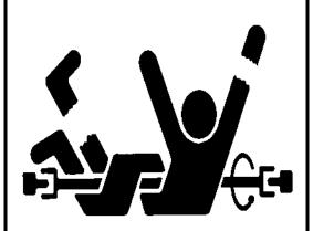
Operating without guards could result in serious injury or death. Machinery in operation can grab, crush, cut, mangle and dismember. Do not operate without adequate guards in place.
