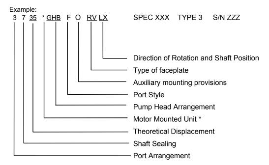
\* The letter (M) may be used in this space indicating the pump is mounted with motor.
