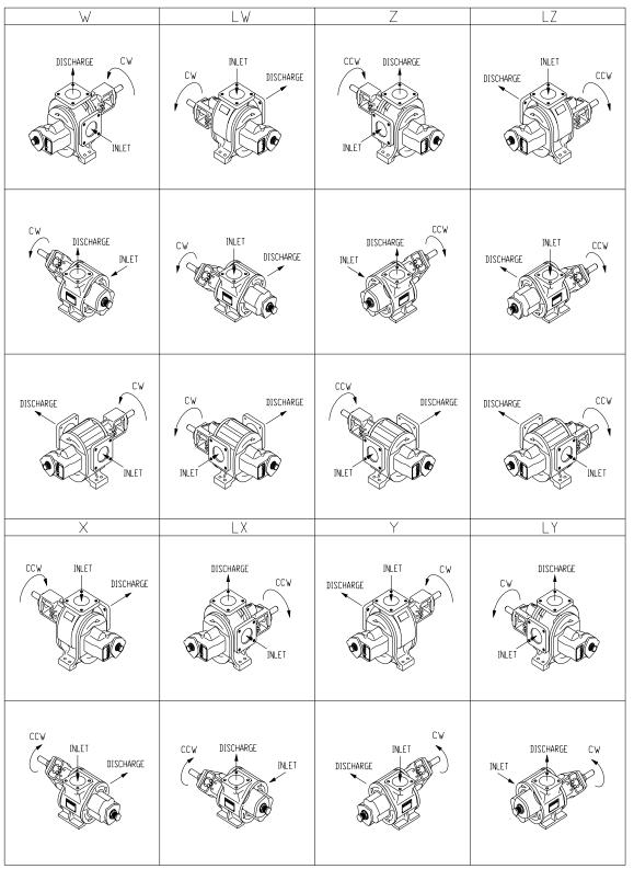
DIRECTION OF ROTATION FOR HB PUMP CONFIGURATIONS USING THE RV STYLE RELIEF VALVE FIGURE 5.4
