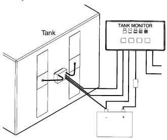
For use on non-conductive tanks (polyethylene, fiberglass, etc.). NOT FOR USE ON FUEL TANKS.
