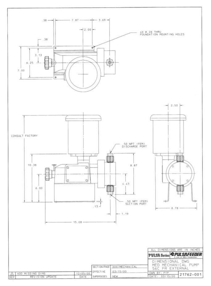
LI4 Medium Mechanical Pump Dimensional Diagram
