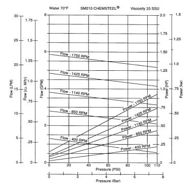
Notes: For continuous service: Plastic / Plastic gear combinations are limited to 50 psi. Metal / Plastic gear combinations are limited to 100 psi.
