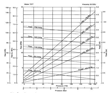
Notes: For continuous service: Plastic / Plastic gear combinations are limited to 50 psi. Metal / Plastic gear combinations are limited to 100 psi. Metal/Metal gear combinations are limited to 150 psi. Horsepower requirements increase for viscous fluids.
