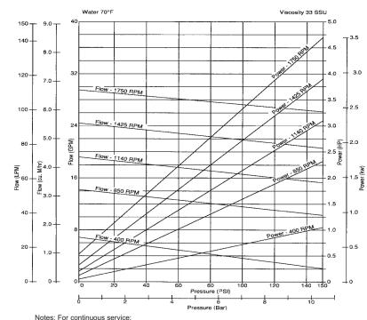
Plastic / Plastic gear combinations are limited to 50 psi. Metal / Plastic gear combinations are limited to 100 psi. Metal/Metal gear combinations are limited to 150 psi Horsepower requirements increase for viscous fluids
