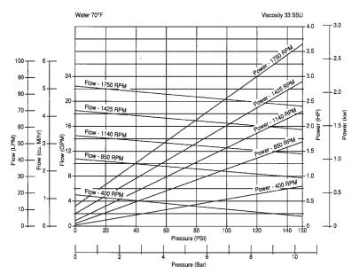
Notes: For continuous service: Plastic / Plastic gear combinations are limited to 50 psi. Metal / Plastic gear combinations are limited to 100 psi. Metal/Metal gear combinations are limited to 150 psi. Horsepower requirements increase for viscous fluids.
