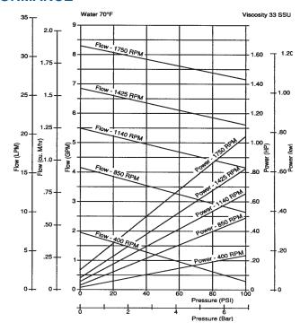
Notes: For continuous service: Plastic / Plastic gear combinations are limited to 50 psi. Metal / Plastic gear combinations are limited to 100 psi. Horsepower requirements increase for viscous fluids.
