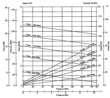
Notes: For continuous service: Plastic / Plastic gear combinations are limited to 50 psi Metal / Plastic gear combinations are limited to 100 psi. Metal/Metal gear combinations are limited to 150 psi. Horsepower requirements increase for viscous fluids.
