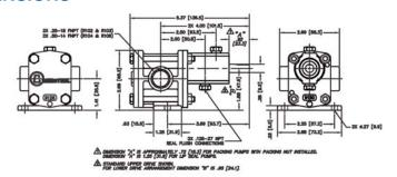
Е G Н J М N 0 R Mechanical Pack Lip Diameter Standard drive Lower drive inches 0.25 0.38 0.92 0.72 1.25 5.36 4.00 3.69 0.63 1.25 0.28 1.88 0.95 2.69 2.69 0.22 2.25 2.88 1.41 millimeters 9.5 23.4 18.3 31.8 136 1 101.6 16.0 31.8 47.6 24 0 68.3 35.8 Notes: Dimension is approximated with packing nut installed
