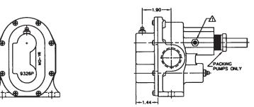
AGREASE FITTINGS (ITEM 17) INSTALLED INTO .125-27 NPT CONNECTIONS.
