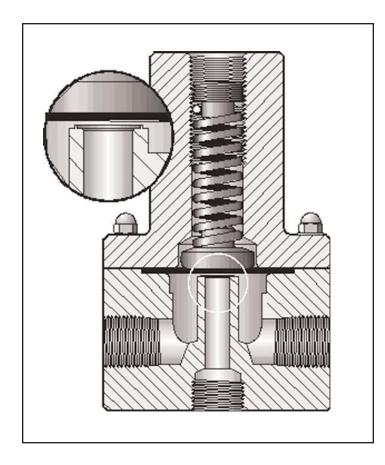
Diaphragm pressure relief valves are designed to protect chemical feed systems from over pressure damage caused by defective equipment or a blockage in the chemical feed line. Robust construction ensures reliability in the rigorous service of municipal and industrial applications. Materials of construction include PVC, 316 SS, and Hastalloy C®. Available in sizes 1/4" through 1".
