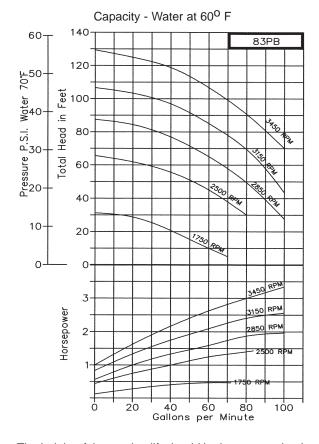
The height of the suction lift should be kept to an absolute minimum and the size of the suction pipe should be equal or larger than the pump inlet port. A foot valve with strainer is recommended a the beginning of the suction line. Self-priming centrifugals must be operated with the shaft in the horizontal position, regular centrifugals may be operated with the shaft horizontal or vertical.
