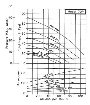
maximum flow. With a throttled discharge, the flow decreases at a greater rate than the pressure increases thereby requiring less horsepower at the higher pressures. This is known as an "unloading" feature of the pump.
