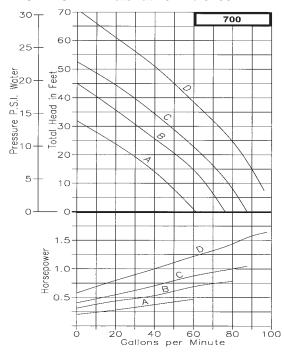
Liquids heavier than water require additional horsepower in direct proportion to the increase in specific gravity. Liquids contaminated with small solids or abrasives can be handled, but a reduction in mechanical seal life must be expected.
