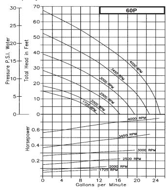
at a greater rate than the pressure increases thereby requiring less horsepower at the higher pressures. This is known as an "unloading" feature of the pump.
