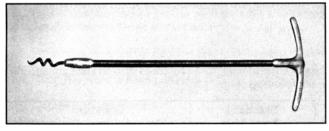
Figure 4-2. Packing Removal Tool
