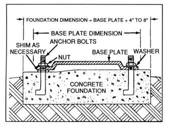
Figure 2-1. Typical Foundation Example
