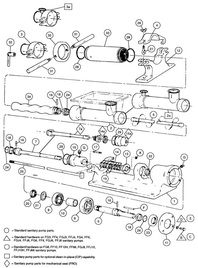
Figure 4-4. Pump Exploded View
