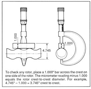
Figure 4-3. Measuring Rotor Dimension
