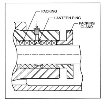
Figure 4-1. Cross Section of Packing Retainer
