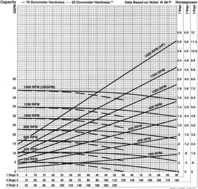
\*\*Std. Nitrile, EPDM, and Fluoroelastomer = 70 Duro. Std. Natural Rubber = 55 Duro.
