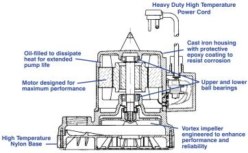
This high temperature version of the 10E Sump/Effluent Pump is capable of pumping up to 200°F liquid. Uses include boiler blow-down pits, rendering plant wash-down sump pits, public utility underground transformer vaults, industrial steam cleaning sump pits, etc. Pumps feature a 1-1/2 discharge, with a lift of 24. Cast iron housing, volute, and relay housing with protective epoxy coating, nylon base and vortex nylon impeller.
