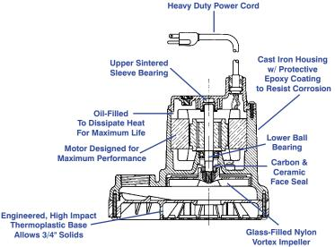
The Model 9E Series De-watering and Effluent pumps are for residential and light to medium commercial use. Pumps feature a 1-1/2" discharge with a lift of 23', glass-filled nylon cover and ABS base.
