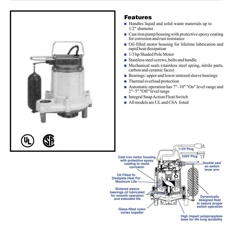
The model 6E Series Sump and Effluent Pumps are for residential and light commercial use. Pumps feature a 1-1/2 FNPT discharge with a lift of 20, polypropylene base and polycarbonate cover.
