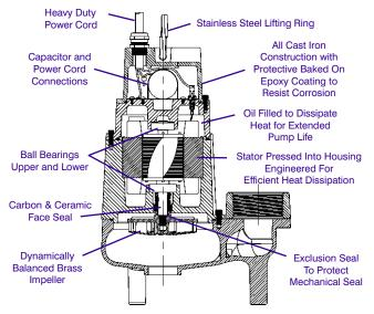
For Residential, Commercial, Industrial and Agricultural use. The Model 20S Series sewage ejector pumps handle liquids and solids up to 2" in diameter. Pumps feature 3" FNPT discharge with a maximum head of 77', heavy duty cast iron construction and stainless steel hardware.
