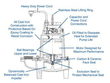
For Residential, Commercial, Industrial and Agricultural use. Pumps feature 3" FNPT discharge with a maximum head of 35', heavy duty cast iron construction and stainless steel hardware.
