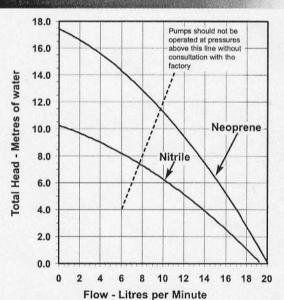
Note: Performance shown is for a new pump, pumping water at 20°C, performance may vary by up to 15%. Consult factory for performance of alternative impeller compounds.
