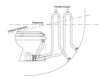
Occasionally, the addition of a vented loop in the inlet hose can cause diminished rinse water flow or poor pump primeability. If this occurs, an electrical air vent solenoid valve (Jabsco Model # 37068-0000) should be added to the air intake of the vented loop assembly and wired in parallel with the toilet pump assembly to close the air supply to the vented loop fitting during the flush cycle (see solenoid valve installation and wiring diagram).
