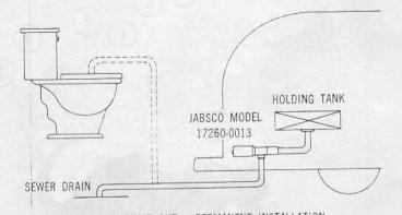
HOLDING TANK PUMP OUT — PERMANENT INSTALLATION
