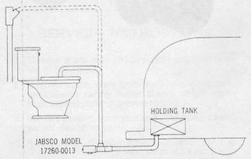
HOLDING TANK PUMP OUT - EXTERNAL CONNECTION
