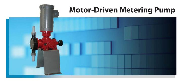
LK Series metering pumps are motor-driven, mechanically actuated diaphragm metering pumps with a maximum capacity of 114 GPH (432 l/h) and a maximum pressure of 225 PSI (1.5 MPa). The LK Series is ideal for chemical feed applications in a wide range of fields, including water treatment, chemical process, agriculture, mining and paper.
