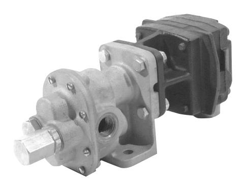
This positive-displacement pump is ideal for de-icing (pre-wet). Combining the pump and motor as a single unit eliminates the need for shaft alignment or Love-Joy® coupling. The unit's compact size allows it to be used in a wide variety of locations and makes it especially attractive for quick, easy retrofit installations.
