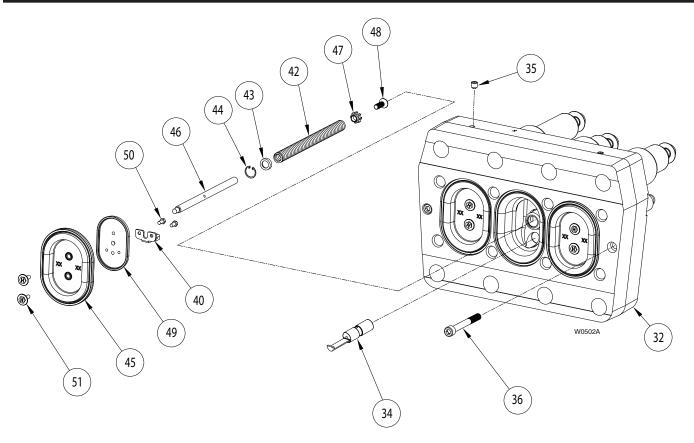
WARNING: Diaphragm plate (32) and assembled parts weigh over 100 pounds (45 kg) and are a two man lift. Use care in handling to prevent personal injury or damage to equipment.
