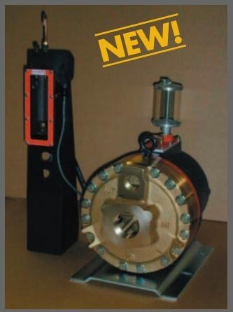
The Hydra-Cell Oil Level Monitoring System utilizes a Murphy Switchgage Model L129CK1. Field proven in the oil industry to detect crank case oil level, the Murphy Switch is well suited to detect oil level for Hydra-Cell pumps such as the D-35 shown here.
