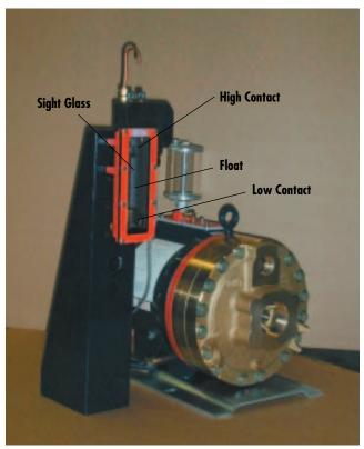
In remote applications such as an oil field or critical applications such as a paper mill, detecting a sudden, radical change in pump oil level can save the pump from severe damage and more importantly, minimize costly interruptions to the process.
