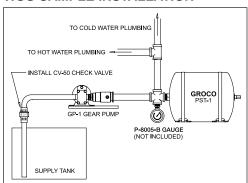
from each outlet, shut it off. When all outlets are closed, the pump will fill the water heater and PST-1 tank (this may take a few minutes) and shut off at 38-40 PSI. Check once again for leaks.
