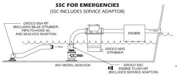
Emergency bilge pumping allows high bilge water to be drawn through open side port and pumped overboard through engine exhaust system.
