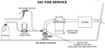
NOTE: SSC may also be installed after the strainer, See SSCV below.
