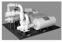
Turn on the AC breaker, and open a faucet to release system pressure. When system pressure drops to approximately 30 PSIG, the AC pump will operate, and will turn off when system pressure reaches 50 PSIG. Note that the DC pump will not operate unless there is no AC power present.
