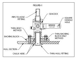
Reversing Handle Rotation: GROCO BV seacocks include the patented user-selectable handle rotation feature. If seacock location does not allow unobstructed handle operation, you may change the rotation direction by relocating the set-screw (Exploded View Item-17). The set-screw may be removed all-together if 180-degree handle rotation is desired.
