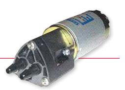
Gear pumps are designed primarily for metering and transfer applications. Their modular design allows a wide variation of flow ranges with a standard parts set. Gear pumps are self-priming and are "constant flow" pumps when RPM and differential pressure are constant. The materials of construction for bodies, gears and seals, provide a wide range of fluid compatibility.
