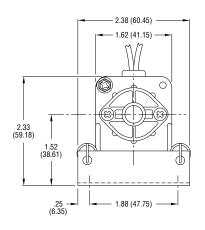
Dimensions in Inches (Dimensions in Millimeters)
