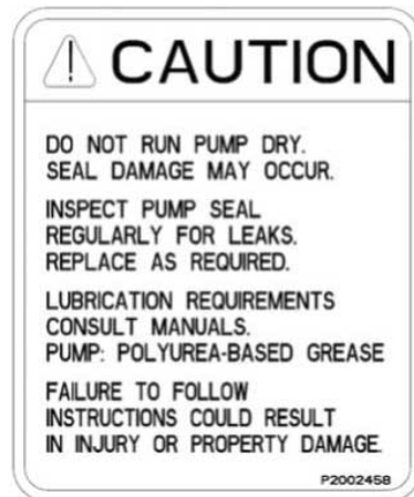
Figure 1: Grease lubricated pumps
