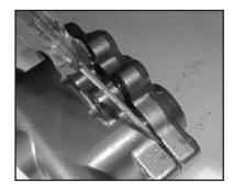
8. Separate the intermediate casing (48) from the valve casing (29)
