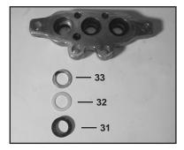
Install the high pressure seal (31), pressure ring (32) and support ring (33-P54W and P58 only) into the intermediate casing (48).
