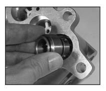
15. Install the seal case (39) with O-rings (40 and/or 40A) into the valve casing (29).
