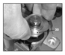
20. Install the pressure rings (30) over the plungers.
