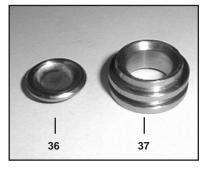
Inspect the valve seat (37) and valve plate (36) for signs of wear or cavitation and replace as necessary.
