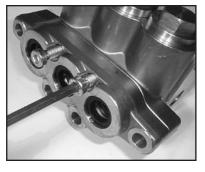
21. Secure the intermediate casing (48) to the valve casing (29) with the inner hexagon screws (46). Torque the screws to 107 in-lbs (12 NM).
