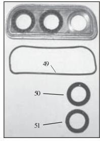
The rear V-sleeve housing (48) may be removed by prying evenly outward with a flat screwdriver. After slipping housing over plunger, inspect rear v-sleeves (50), support rings (51) and O-ring (49) and replace as necessary.
