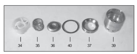
7. Inspect and clean the valve assembly parts. If pitted or worn, replace inlet valve seats (37), valve plates (36), spring (35) and spring retainers (34). Reinsert items 34-38 into valve adapter (39).
