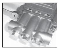
Drain the oil from the pump. Turn the pump over to remove the two manifold stud nuts (46) with a 17mm wrench.
