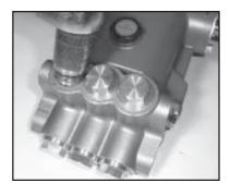
1. With a 22mm socket, remove the three discharge (43) and three inlet (41) manifold plugs. Check o-rings (42 & 44) for wear and replace as necessary.
