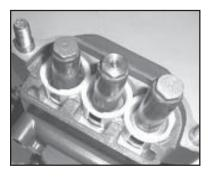
10.Inspect ceramic plunger (24A) tips for wear. If necessary, replacement of the ceramic plungers may be accomplished by removing the plunger bolt assemblies (24B and 24C) with a 13mm wrench. Ceramic plungers should now slide off the stainless steel plunger base (22). Excessive resistance to plunger removal may be overcome by heating the stainless steel plunger base. This will melt any excess loc-tite beneath the ceramic plunger allowing easy removal.
