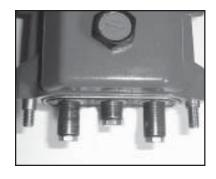
13. Before replacing pump manifold (29), first rotate crankshaft (18) until two outside plungers (24A) extend evenly forward. Next lubricate rear v-sleeves (50) and support ring (51) in the rear v-sleeve housing (48) and slide housing over plungers. Lubricate ceramic plungers with a light film of oil. Carefully and evenly slide manifold over plungers and press manifold firmly against crankcase (1). Replace manifold stud bolts (45), washers (47) and nut (46) and tighten to 35 ft.-lbs.
