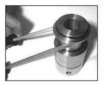
Remove seal case (37) from seal sleeve (35).
