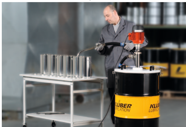
Filling of high-temperature lubricating grease.
