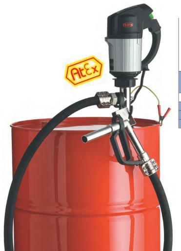
Delivery rate max. 200 l/min, delivery head max. 9,5 m.\* When using the pump with a discharge hose and a hand tap, the delivery rate will be approx. 50 l/min.
