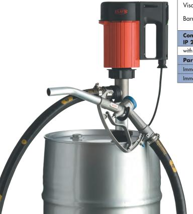
Delivery rate max. 220 l/min, delivery head max. 12 m.\* When using the pump with a discharge hose and a hand tap, the delivery rate will be approx. 80 l/min.
