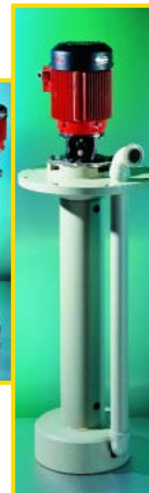
Type F 706: 4 different sizes, sealless design with sleeve bearing, immersion length up to 2000 mm
