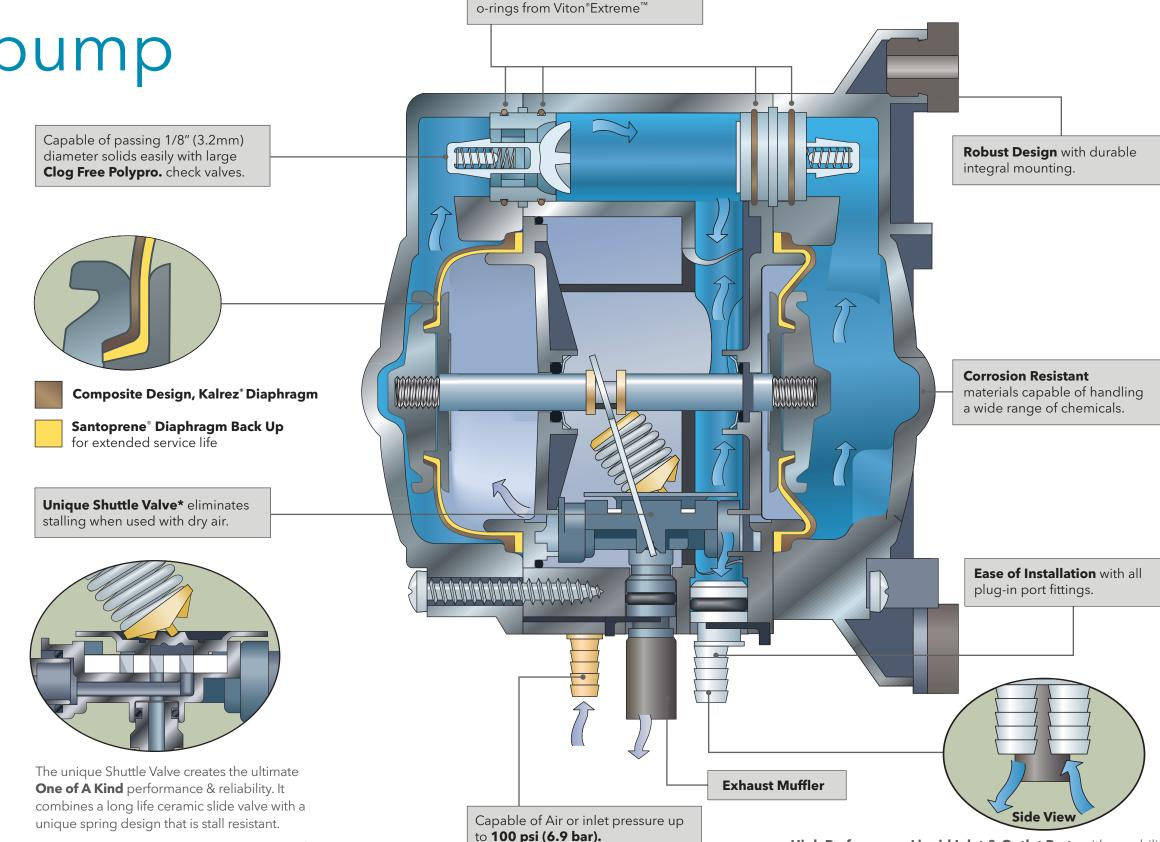
High Performance Liquid Inlet & Outlet Ports with capability
