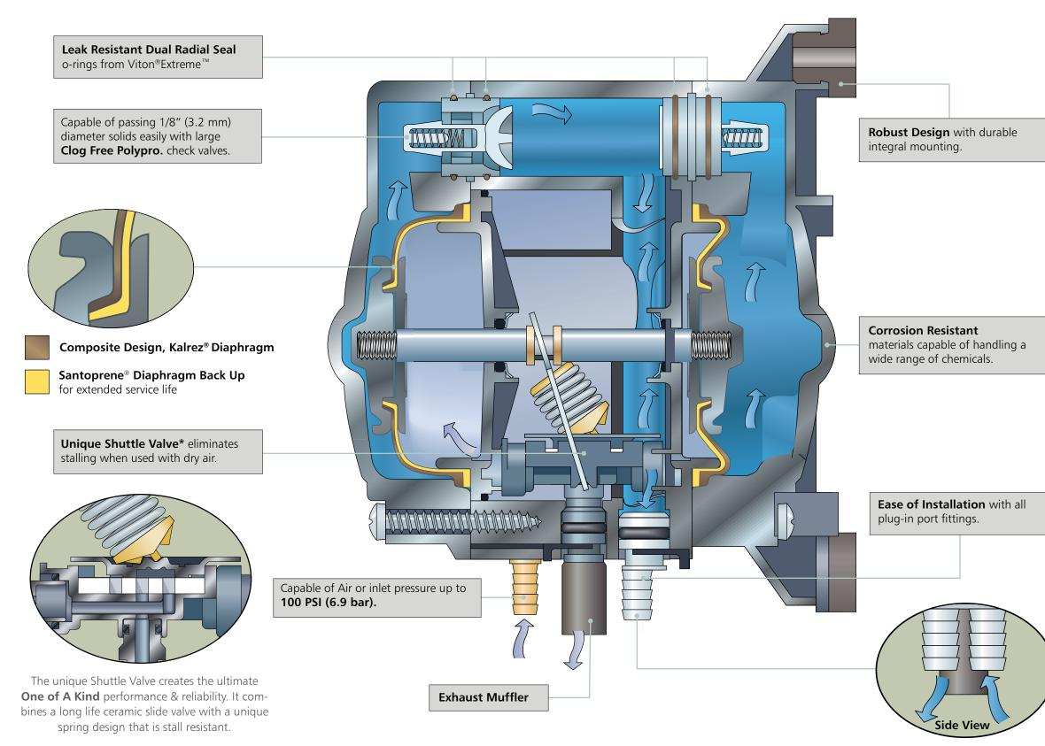
**High Performance Liquid Inlet & Outlet Ports** with capability of supplying flow rate to 5 GPM (18.9  $\ell$ /min.).
